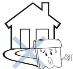
If this water purifier is used outdoors, it can lead to accelerated aging of the water purifier pipes and parts, which can cause leaking or machine failure.
